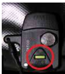
UML Pro Sensor mechanism indicating the cylinder has not been used.
