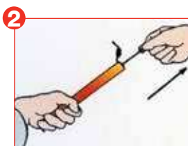
Pull the top. The flare ignites after 2 second delay
